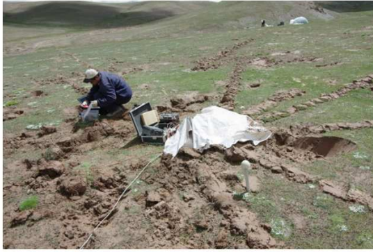
Figure 7.6: Electrodes layout scheme characterizing the star configuration.
