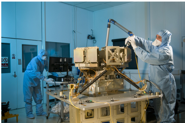
Figure 4: MIRI being aligned at the Rutherford Appleton Laboratory prior to its shipment to NASA Goddard. The emphasis at DIAS has now shifted to development of MIRI data analysis software and improved pipeline calibration.
