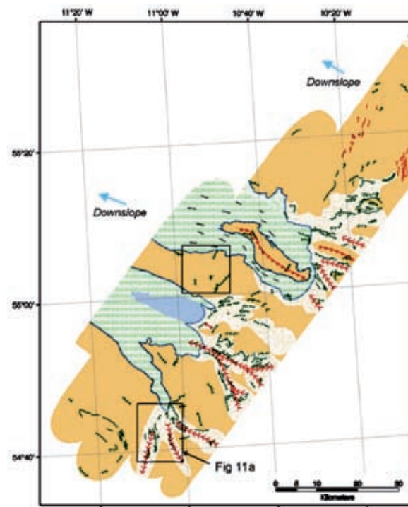
Figure 4.5.1: Example of TOBI interpretation from the eastern side of the Rockall Trough, showing two large canyon systems. Red lines indicate canyon axes and ridges and green areas indicate sediment aprons.
